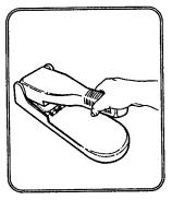
Grasp the flower press handle and bring the top down onto the design plate. Press down on the handle. Swing the flower press top up and remove the design plate.
