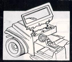
7. To assemble windshield, insert tabs into slots in hood and push down until pegs go into holes. Windshield can be removed for Dino-Damage.
