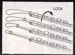
Boom can be adjusted to different lengths, and locked into position.
