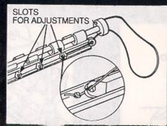
String can be adjusted to 5 different loop sizes.
