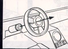
2. Steering wheel snaps onto steering column.
