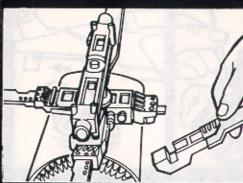
5. Align each rotor blade with pegs on prop and snap down into position.
