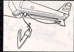
**3.** Tie cable onto fin. Feed cable under crossbar. Tie cable onto hook.
