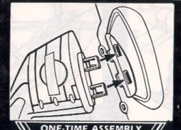
2. Press landing skids into slots on both sides of copter.
