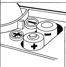
CAUTION: To avoid battery leakage, (1) Be sure to insert the batteries correctly and follow the toy and battery manufacturer's instructions. (2) Do not mix old and new batteries or alkaline, standard (carbon-zinc) or rechargeable batteries. (3) Always remove exhausted or dead batteries from the product.
