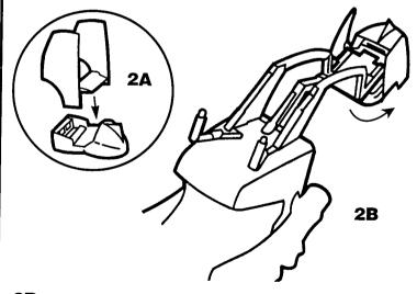
**2B.** Then insert the front arms of the vehicle into the assembled nose piece. Lower the arms to snap them into the nose piece.
